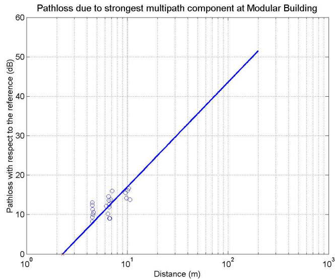
Figure 5.2 Pathloss of Strongest Multipath Component in Modular Building
