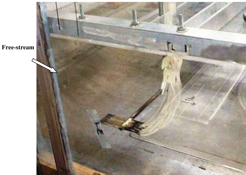
Figure 2.3: The pressure rake set to measure the sidewall boundary layer in the Virginia Polytechnic Institute and State University Boundary Layer Wind Tunnel
