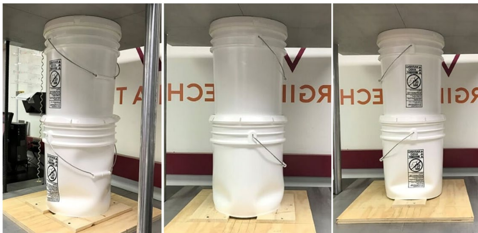
Image 6. Pail failure modes on simulated pallet deckboards.
