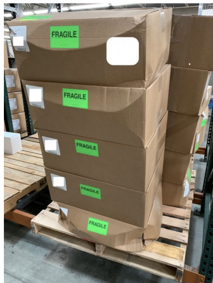
Image 2. Showing sidewall buckling of corrugated boxes on a less stiff pallet.
