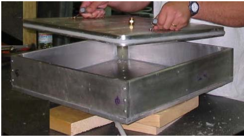
Figure 3-8. Transverse permeability specimen holder.
