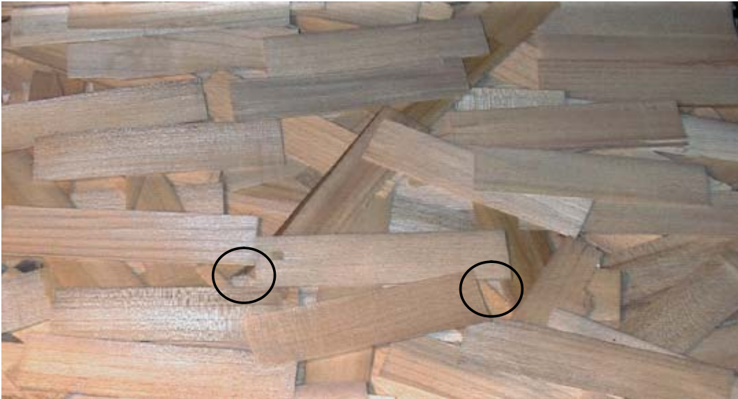
Figure 4-9. Between flake openings available for transverse flow.
