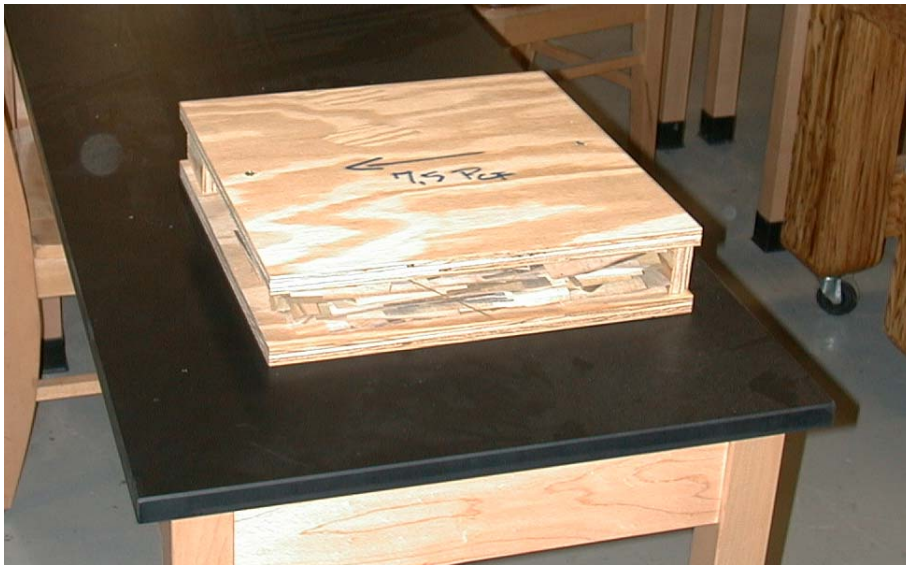
Figure 3-4. OSB sample mat restrained by plywood.
