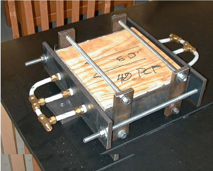
Figure 3-6. In-plane permeability specimen holder.
