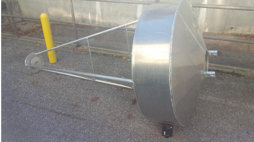
Figure 2-14 The manufactured floating buoy for the self-reactive point absorber
