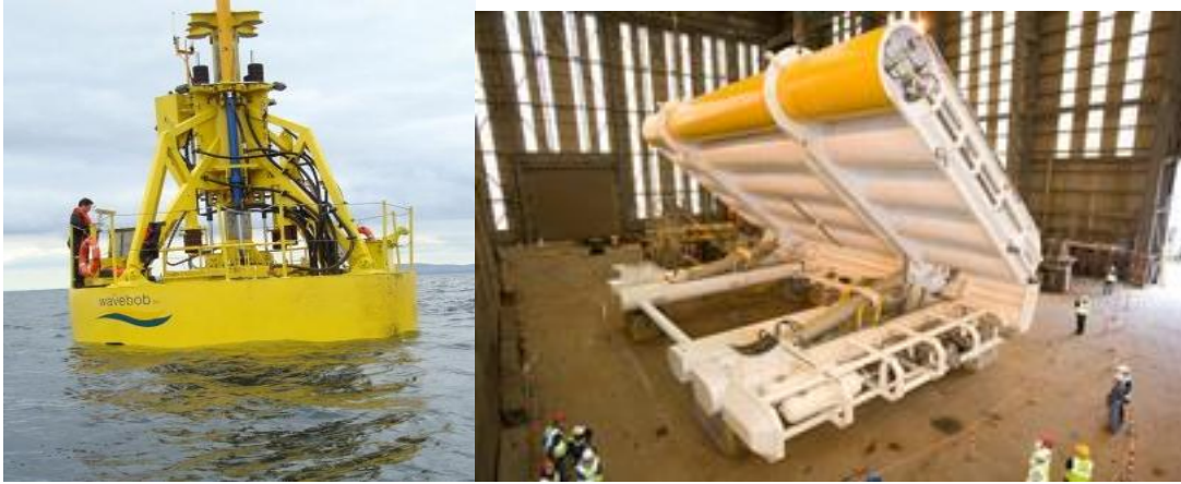
Figure 1-4 Left: Wavebob, a typical point absorber; Right: Oyster, a wave surge device designed for shallow water use
