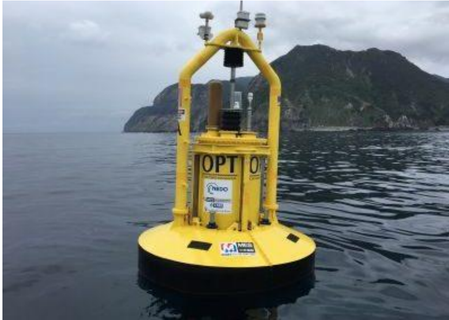
Figure 1-7 An Ocean Power Technology's PB3 power buoy is under sea trial
