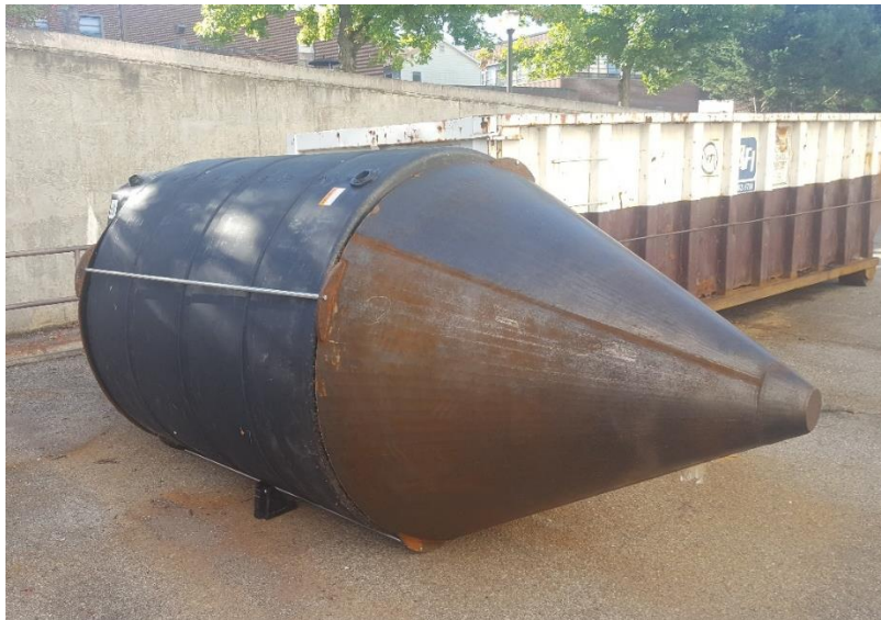
Figure 2-15 The manufactured submerged body for the self-reactive point absorber
