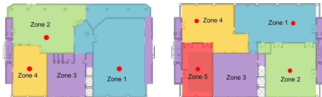
Fig. 2 Floor plans on Floors 1–2 (left) and Floors 3–7 (right). Red dots illustrate the approximate locations of multi-sensors on each floor. Note that Floor 1 has no sensor.
