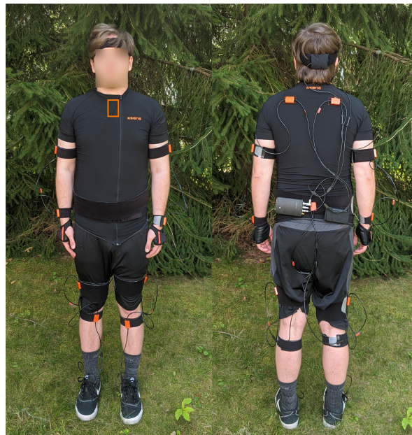
Figure 3. Location and placement of the inertial sensors in this study using the guidelines set by XSens. The sensors were also wrapped with excess webbing, as shown in Figure 2c (not shown in this photo for ease of seeing the sensor locations). Some participants used custom shirts with Velcro patches when the XSens shirt was too small. The wires along the back and limbs were secured and bundled together to make sure they did not catch on objects. Note that there is a sensor on the sternum (indicated by the orange box), but it is inside a pocket on the front of the shirt so is not visible in the photo.
