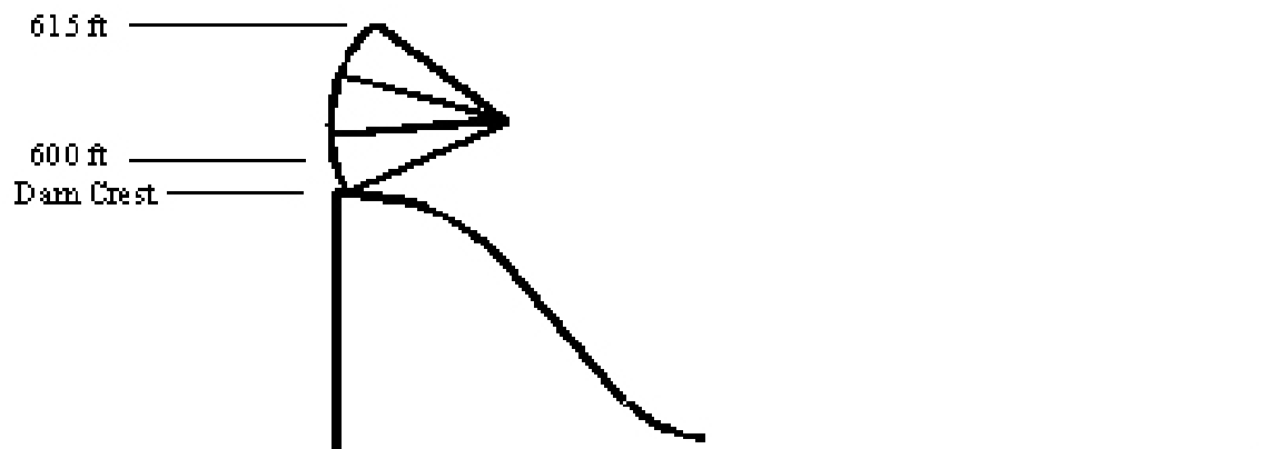
Figure 4-6. Lower Reservoir Gate
