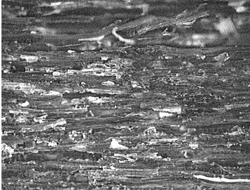
Figure J.1: Image 1 of a boiled pMDI bonded hygro-thermal treated sample (taken @ 5x, 1626 x 1235 \mu\text{m} field of view).
