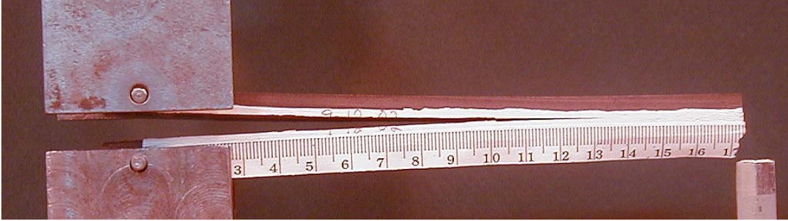
Figure 3.14: A fracture sample in testing which illustrates the use of white correction fluid and a ruler.
