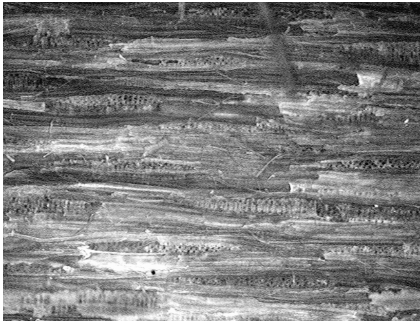
Figure F.18: : Image 6 of a PF-film bonded densified sample (taken @ 5x, 1626 x 1235 \mu\text{m} field of view).
