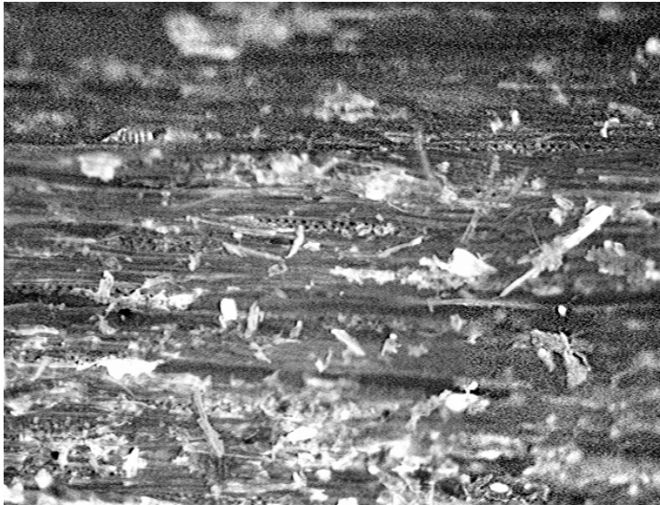
Figure 4.10: Reflected light microscope image (taken @ 5 x, 1626 x 1235 \mu\text{m} field of view) of a failed bondline surface of a boiled hygro-thermal fracture sample bonded with pMDI.
