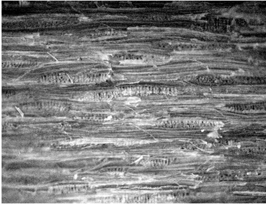
Figure F.5: Image 1 of non-bonded densified yellow-poplar (taken @ 5x, 1626 x 1235 \mu\text{m} field of view).
