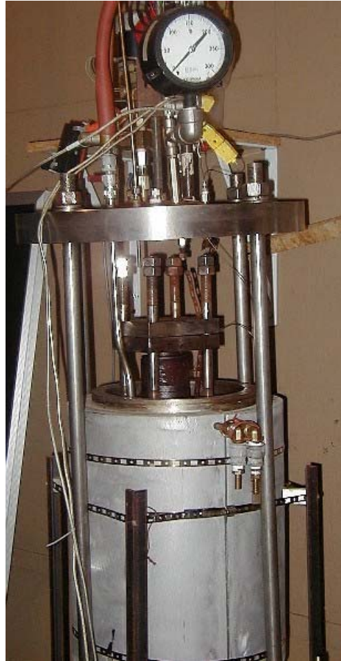
Figure 3.6: Pressure vessel used for wood treatment.
