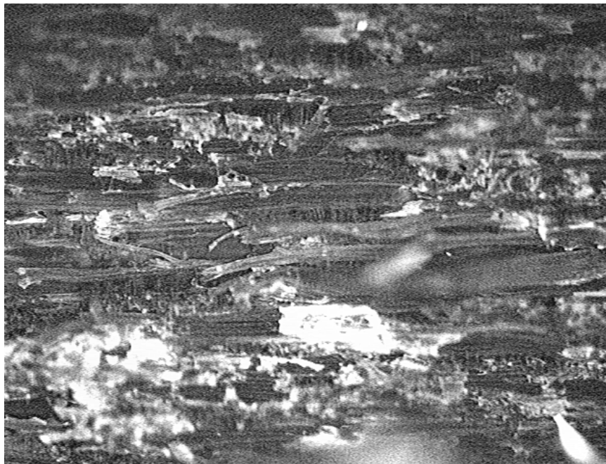
Figure J.4: Image 4 of a boiled pMDI bonded hygro-thermal treated sample (taken @ 5x, 1626 x 1235 \mu\text{m} field of view).
