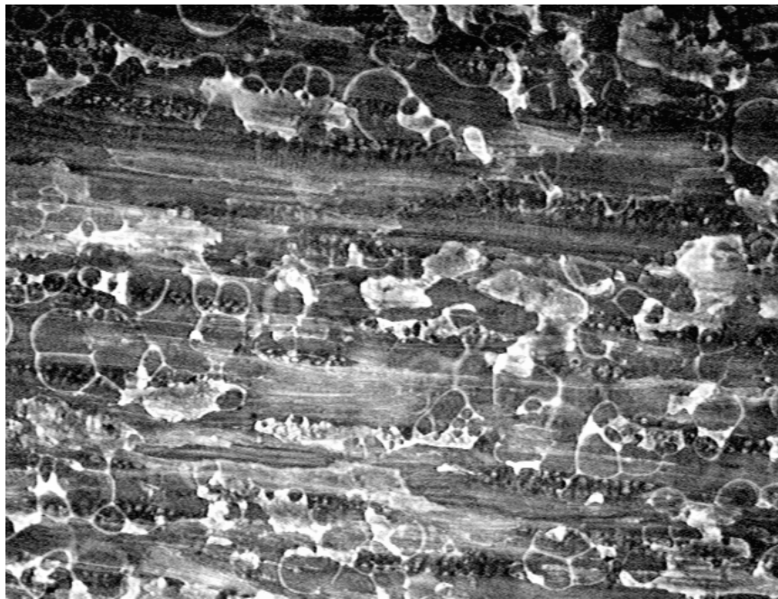
Figure J.6: Image 2 of a boiled pMDI bonded densified sample (taken @ 5x, 1626 x 1235 \mu\text{m} field of view).
