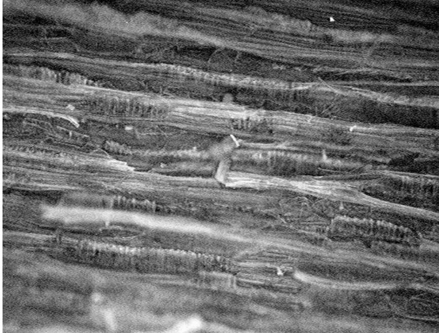
Figure F.3: Image 1 of non-bonded hygro-thermally treated yellow-poplar (taken @ 5x, 1626 x 1235 \mu\text{m} field of view).
