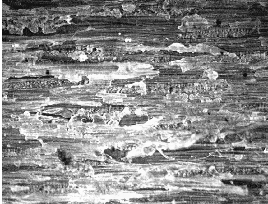
Figure G.3: Image 1 of a pMDI bonded hygro-thermal treated sample (taken @ 5x, 1626 x 1235 \mu\text{m} field of view).
