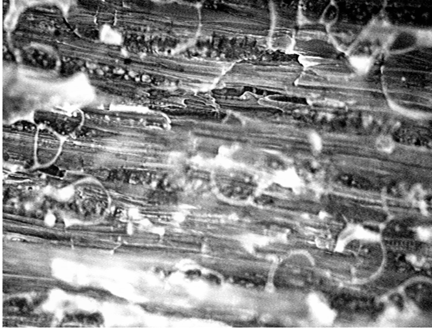
Figure J.7: Image 3 of a boiled pMDI bonded densified sample (taken @ 10x, 827 x 628 \mu\text{m} field of view).
