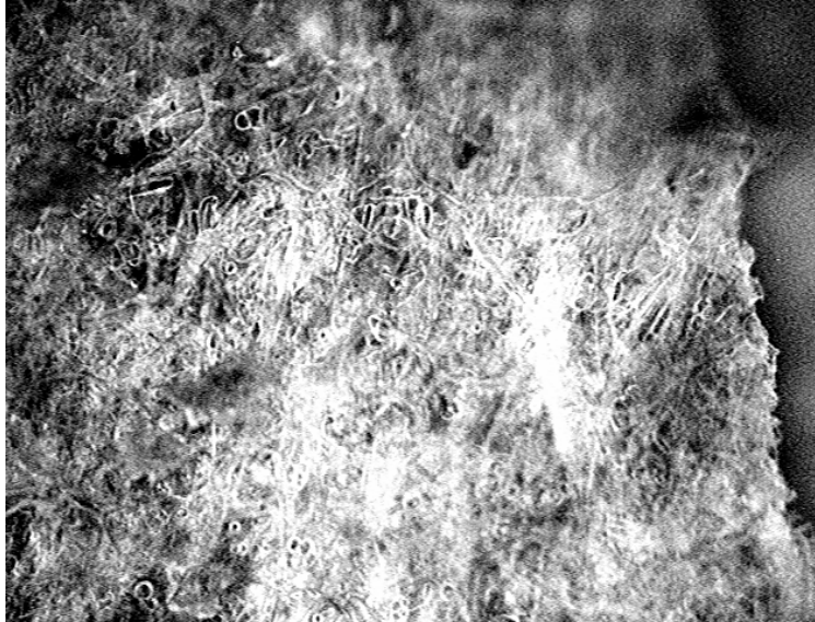
Figure 4.7: Reflected light microscope image (taken @ 5 x, 1626 x 1235 \mu\text{m} field of view) of a failed bondline surface of a boiled densified fracture sample bonded with PF-film.
