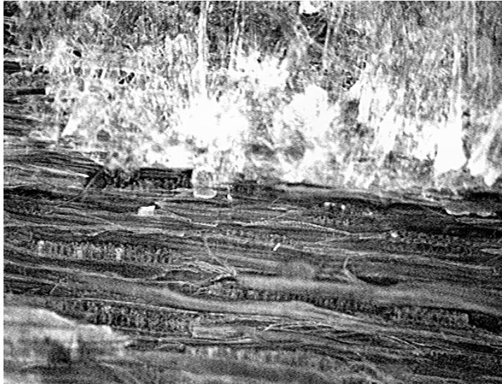
Figure 3.24: Reflected light microscope image (taken @ 5 x, 1626 x 1235 \mu\text{m} field of view) of a failed bondline for a hydro-thermally treated fracture sample bonded with PF-film.
