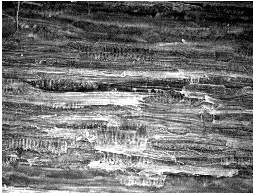
Figure G.6: Image 1 of a pMDI bonded densified sample (taken @ 5x, 1626 x 1235 \mu\text{m} field of view).
