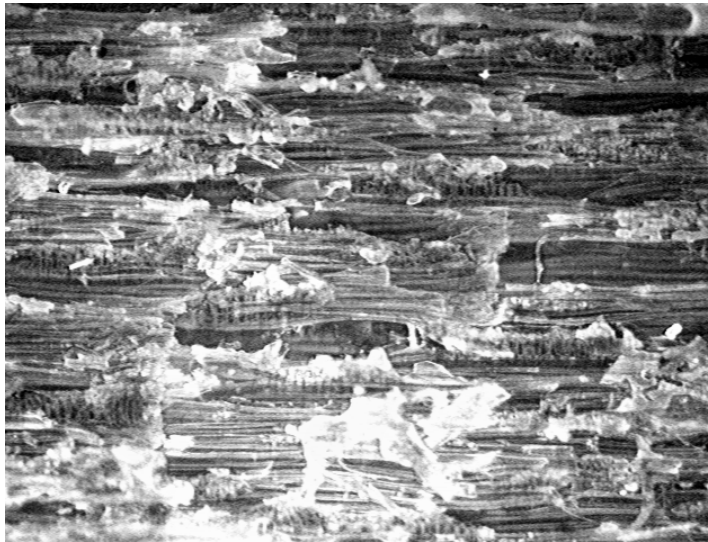
Figure 3.30: Reflected light microscope image (taken @ 5 x, 1626 x 1235 \mu\text{m} field of view) of a failed bondline surface for a hygro-thermal fracture sample bonded with pMDI.
