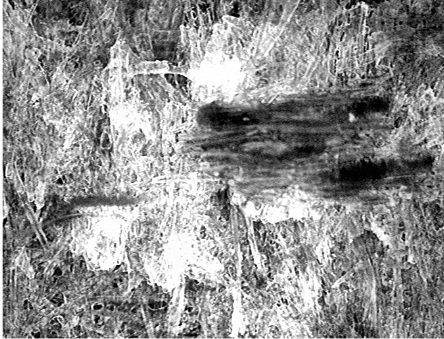
Figure F.9: Image 1 of a PF-film bonded hygro-thermal treated sample (taken @ 5x, 1626 x 1235 \mu\text{m} field of view).
