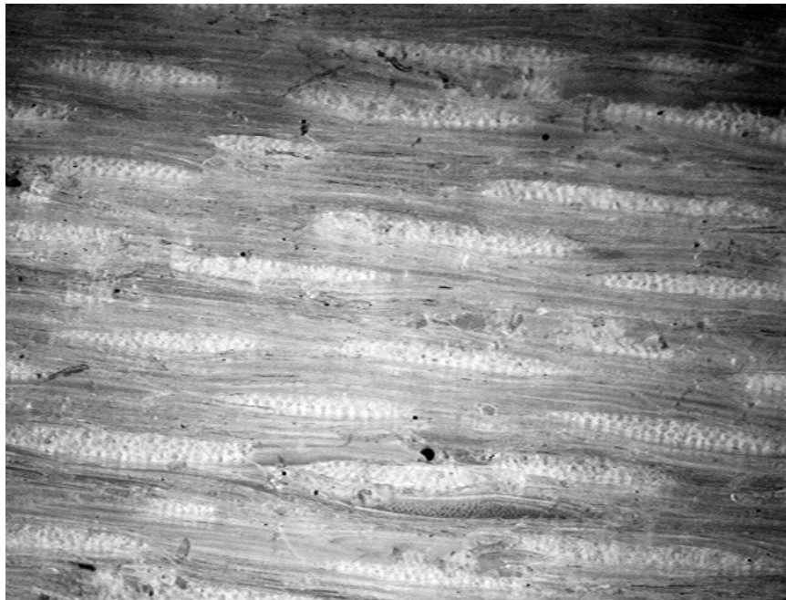
Figure F.2: Image 2 of non-bonded control yellow-poplar (taken @ 5x, 1626 x 1235 \mu\text{m} field of view).
