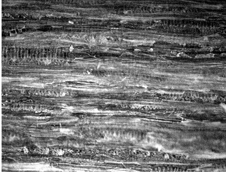
Figure G.7: Image 2 of a pMDI bonded densified sample (taken @ 5x, 1626 x 1235 \mu\text{m} field of view).
