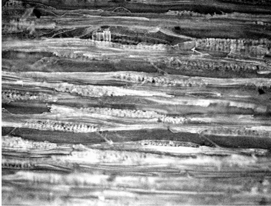
Figure J.5: Image 1 of a boiled pMDI bonded densified sample (taken @ 5x, 1626 x 1235 \mu\text{m} field of view).
