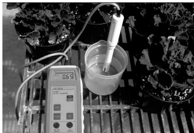
Figure 2. Portable electrical conductivity (EC) meters can be used to measure the EC of the dilute fertilizer solution to verify that the injector is working within the expected range. Compare the EC of the solution to that recommended on the fertilizer bag (Fig. 3) or the fertilizer label.
