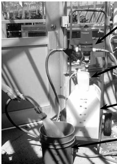
Figure 1. Fertilizer injectors draw fertilizer stock solution from the stock tank (A) and meter it out through the injector (B) at a specified ratio of stock to irrigation water when the irrigation water is flowing. This specified ratio makes up the injector ratio. Checking the calibration of a fertilizer injector involves measuring the amount of “stock” (C) taken up by the injector as a measured amount of irrigation water flows through the injector and is collected in a calibrated container (D).
