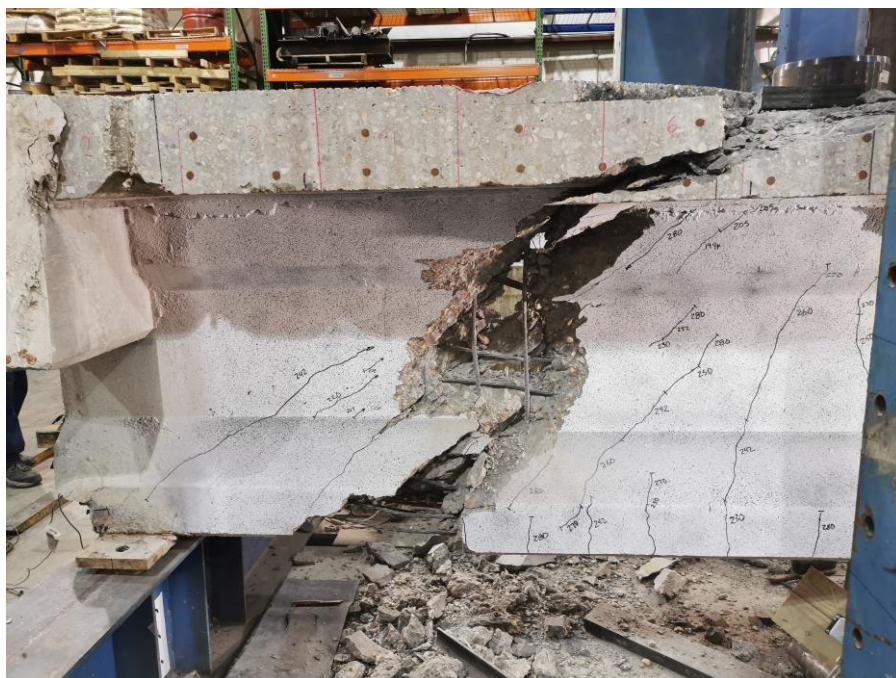
Figure 51 Failure mode for the second Lesner test (Web crushing)
