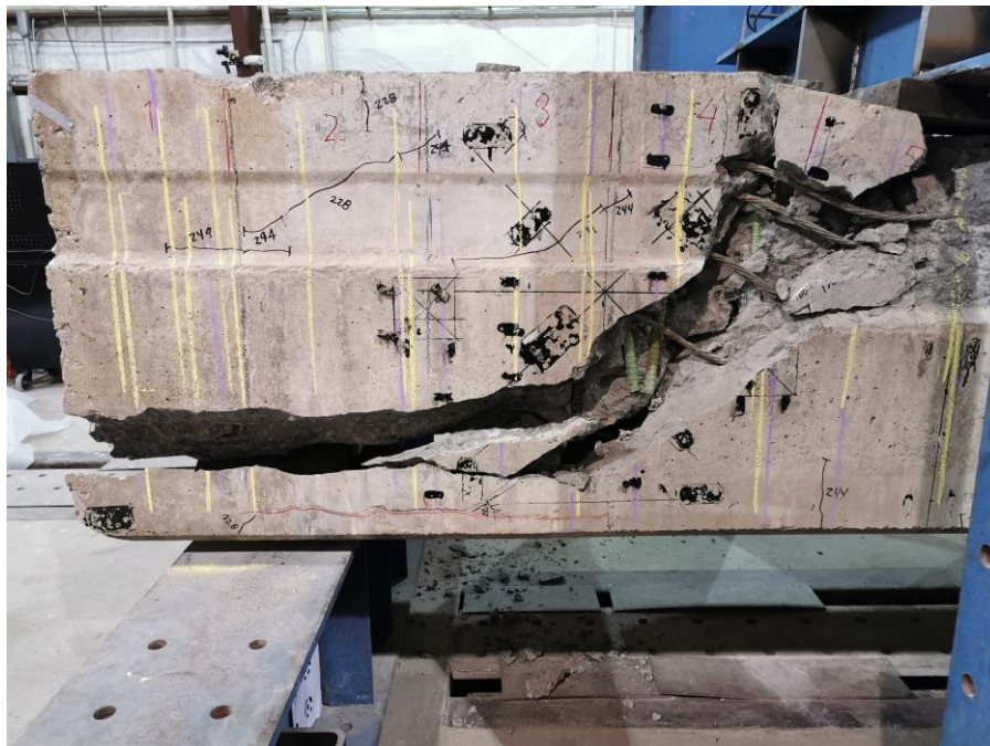
Figure 54 Failure mode for the first Aden test (Diagonal tension)
