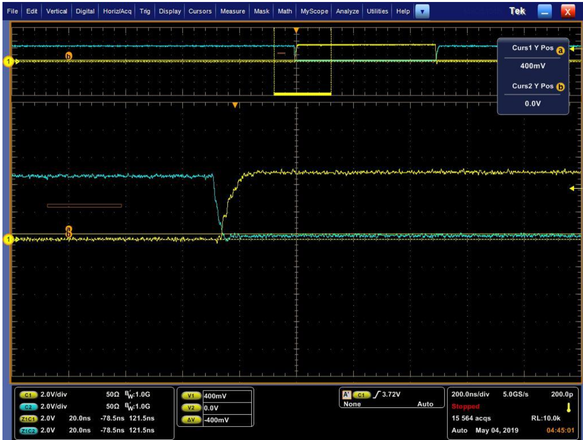
Figure 5.17 - Low Side Gate Signal
