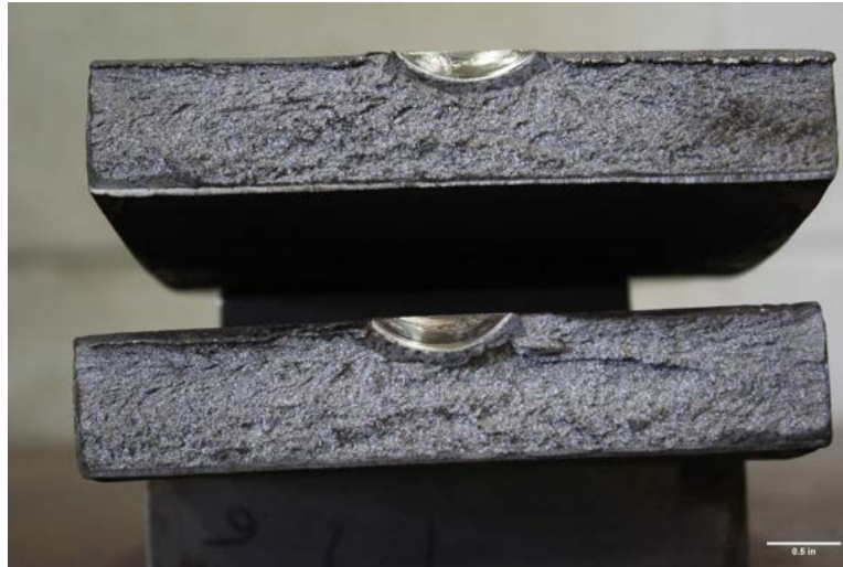
Figure V.45. Fracture surfaces of W36-0.25N-T100-R11.01.
