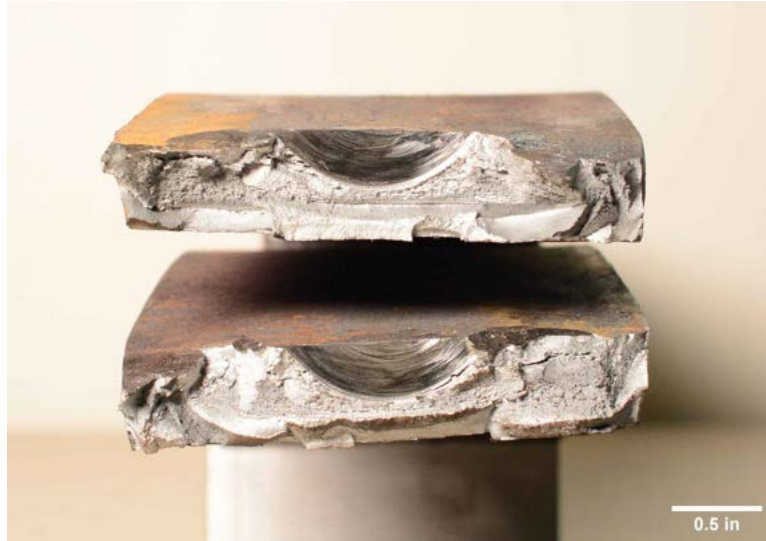
Figure V.54. Fracture surfaces of W24-0.375N-T59-R11.02.
