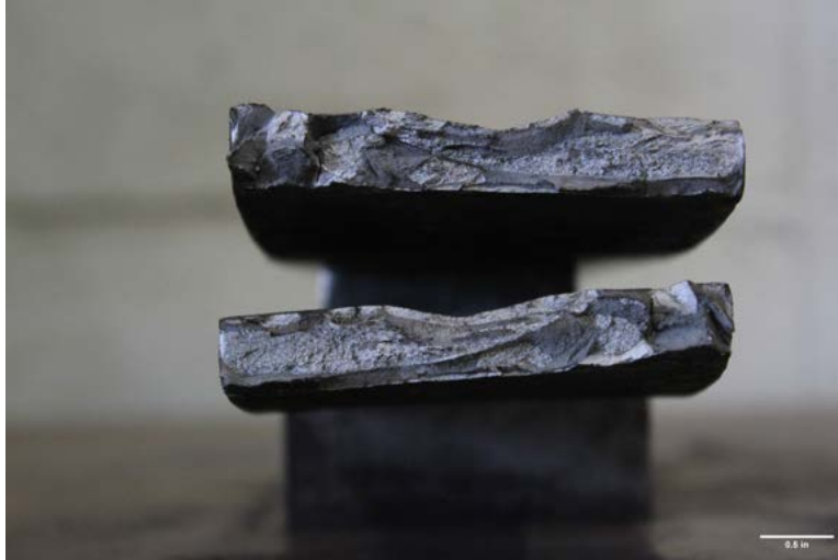
Figure V.4. Fracture surfaces of W24-0.125NGT-T50-R11.02.
