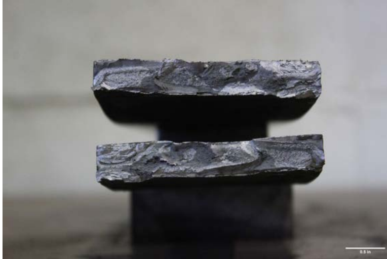
Figure V.67. Fracture surfaces of W24-STEEL-T50-R11.02.
