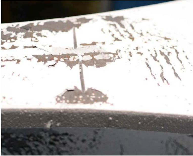
Figure 6.21. Fracture initiation in the bottom of a notch.
