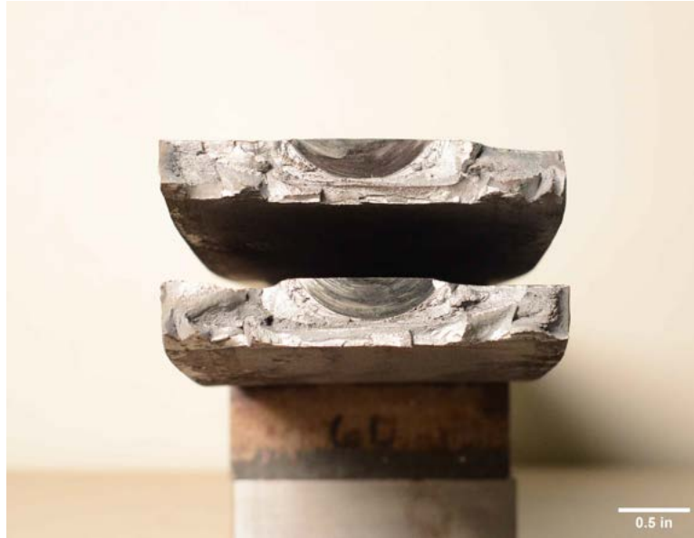
Figure V.48. Fracture surfaces of W24-0.375N-T50-R11.01.
