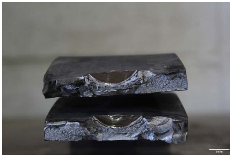
Figure V.34. Fracture surfaces of W24-0.25N-T50-R11.02.
