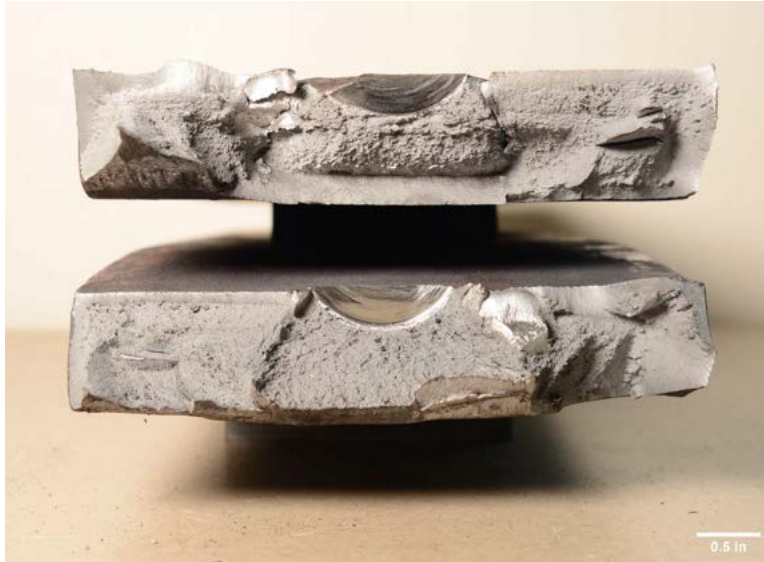
Figure V.61. Fracture surfaces of W36-0.375N-T100-R11.02.
