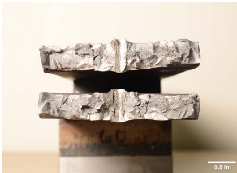
Figure V.85. Fracture surfaces of W24-PAF-T50-R11.02.
