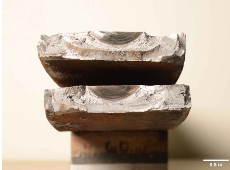
Figure V.52. Fracture surfaces of W24-0.375N-T59-R11.01.
