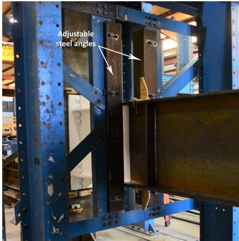
Figure 3.3. Beam lateral bracing with adjustable steel angles.
