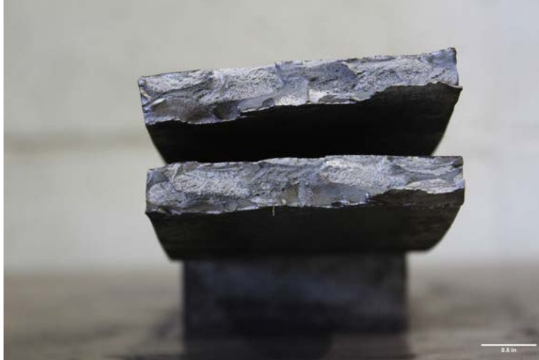
Figure V.69. Fracture surfaces of W24-STEEL-T50-R11.03.
