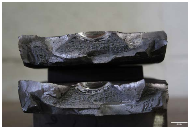
Figure V.42. Fracture surfaces of W36-0.25N-T94-R11.01.
