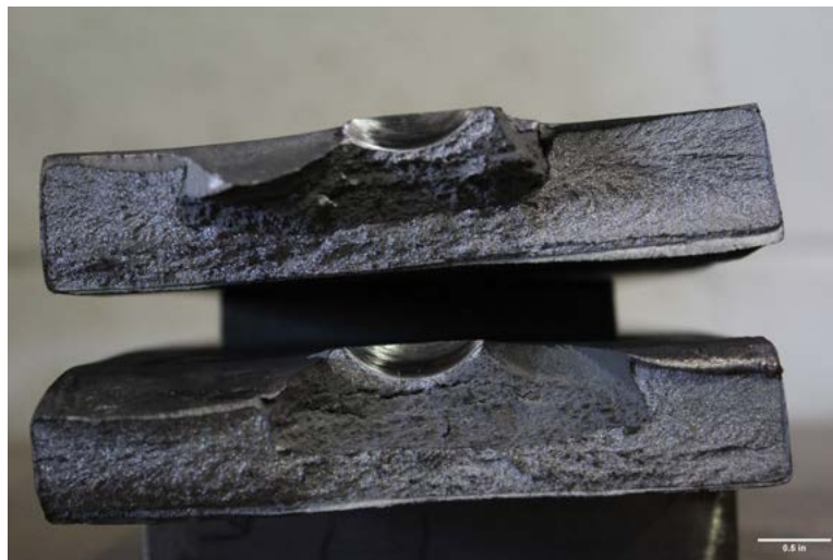
Figure V.46. Fracture surfaces of W36-0.25N-T100-R11.02.
