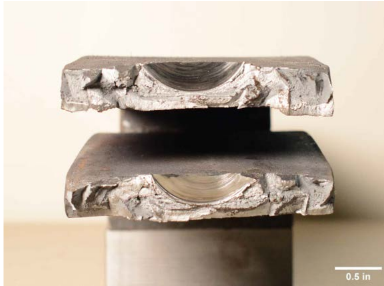
Figure V.50. Fracture surfaces of W24-0.375N-T50-R11.02.
