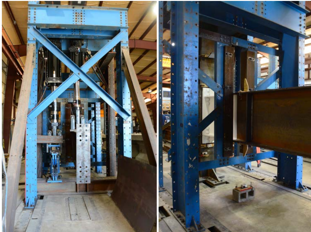
(a) Actuator frame viewed from the south end. (b) Bracing frame viewed from the south end.
