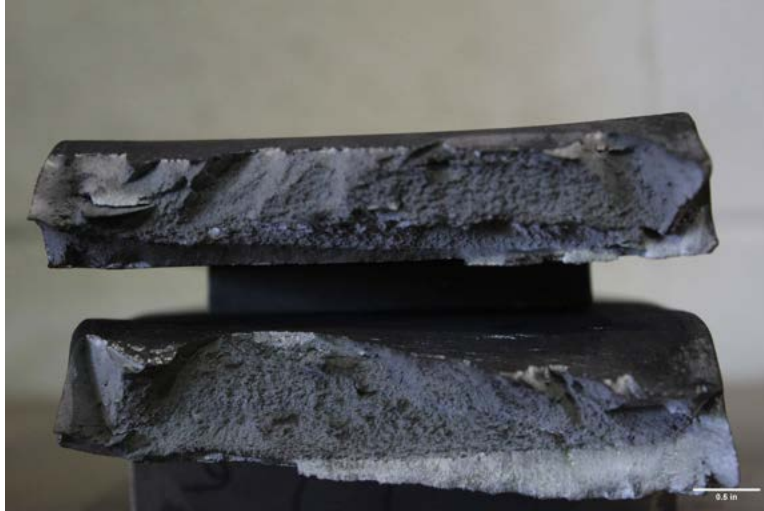
Figure V.73. Fracture surfaces of W36-STEEL-T100-R11.02.
