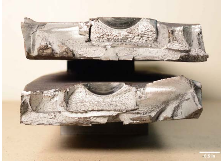
Figure V.58. Fracture surfaces of W36-0.375N-T94-R11.02.
