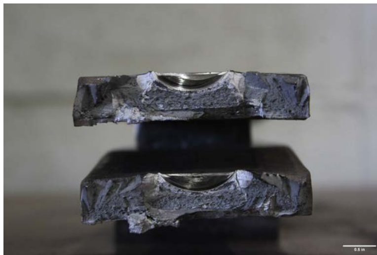
Figure V.40. Fracture surfaces of W24-0.25N-T59-R11.03.
