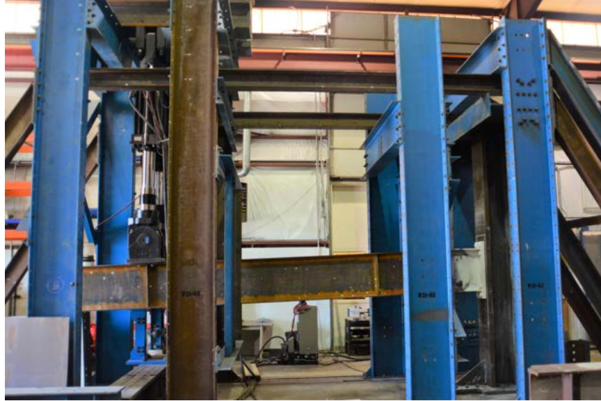
Figure 3.2. Test setup for full-scale moment connections.
