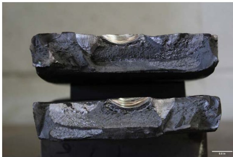
Figure V.44. Fracture surfaces of W36-0.25N-T94-R11.02.
