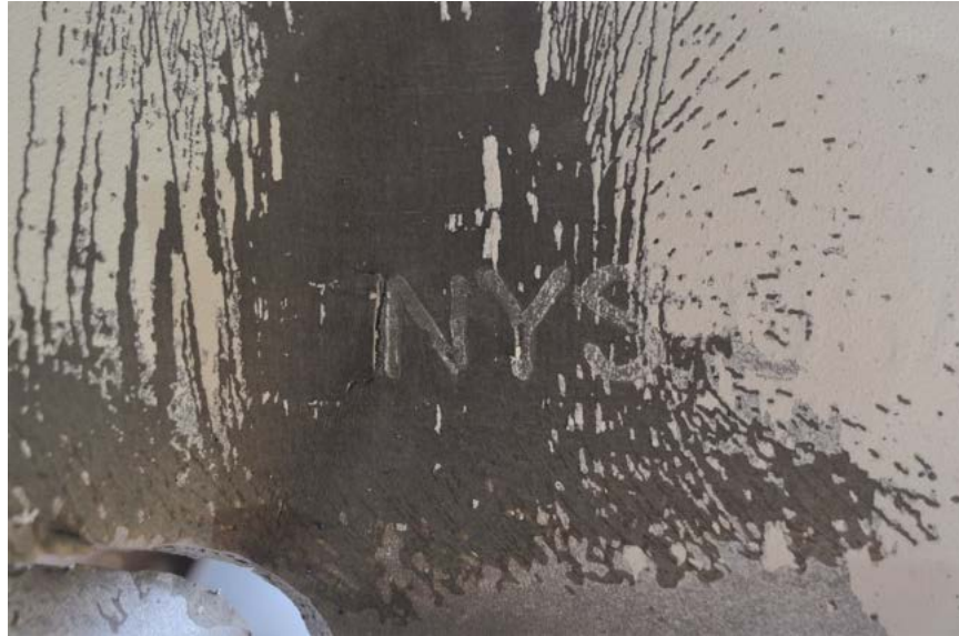
Figure 6.4. Web fracture at a rolling mill stamp on W24RBS-0.125NGT-T59.
