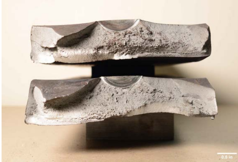
Figure V.60. Fracture surfaces of W36-0.375N-T100-R11.01.
