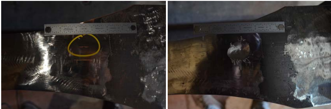
(a) Surface crack.
