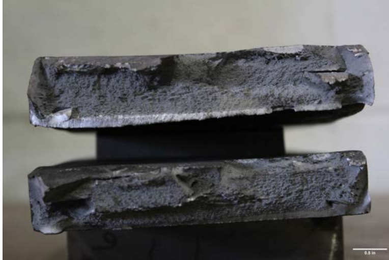
Figure V.71. Fracture surfaces of W36-STEEL-T100-R11.01.
