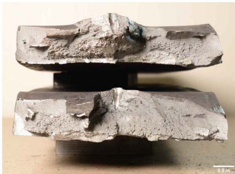
Figure V.95. Fracture surfaces of W36-PAF-T100-R11.01.
