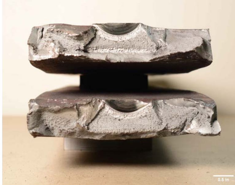
Figure V.56. Fracture surfaces of W36-0.375N-T94-R11.01.
