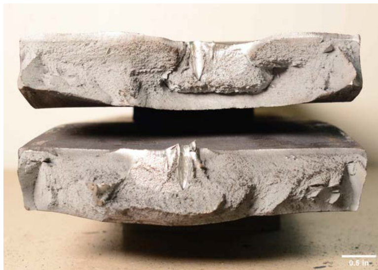
Figure V.97. Fracture surfaces of W36-PAF-T100-R11.02.
