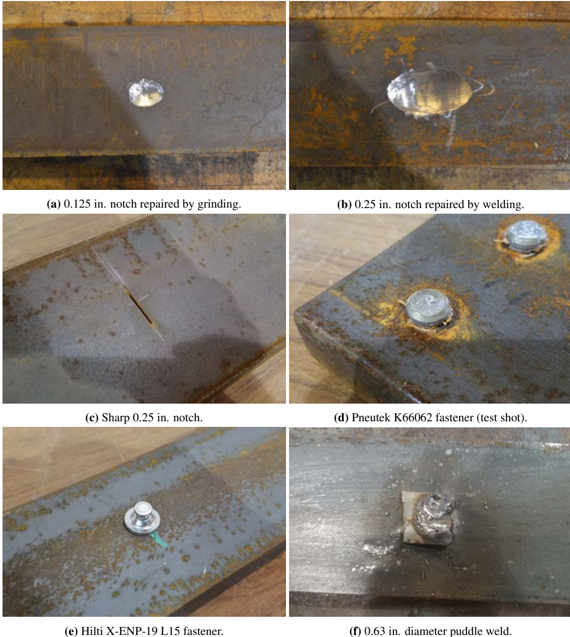
Figure 3.16. Bend coupons with various artifacts.
