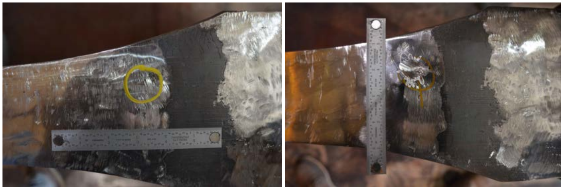
(a) Surface crack.
