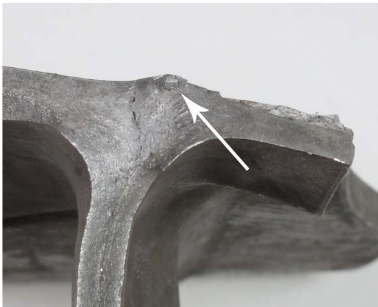
Figure 6.44. Subsurface-origin fatigue fracture on a full-scale specimen with welded artifacts.
