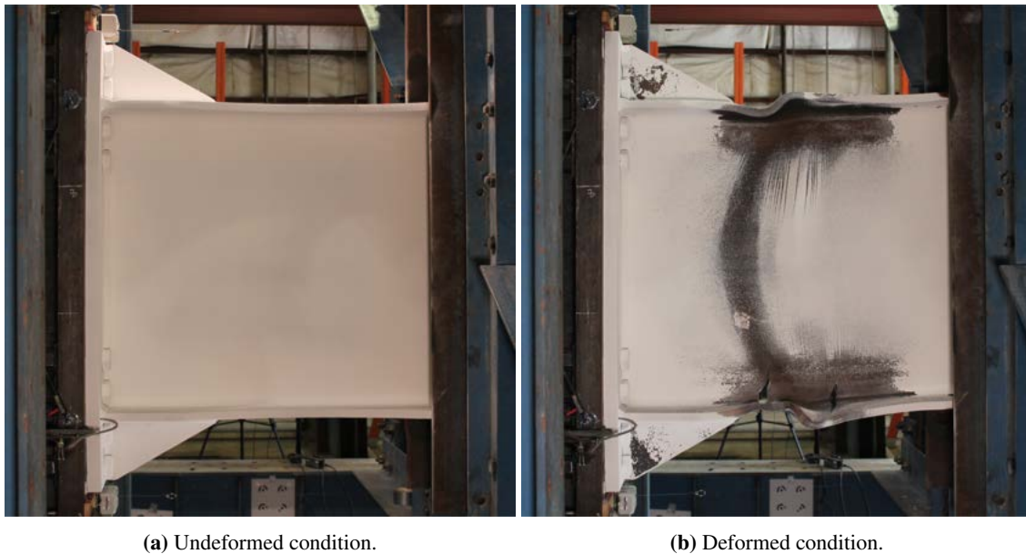
Figure 6.15. Undeformed and deformed conditions of W36RBS-0.25NGTW-T94.
