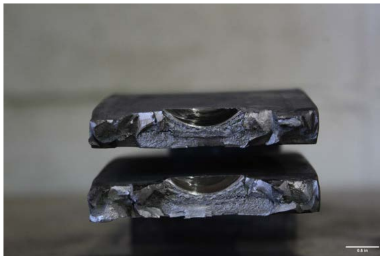
Figure V.36. Fracture surfaces of W24-0.25N-T50-R11.03.
