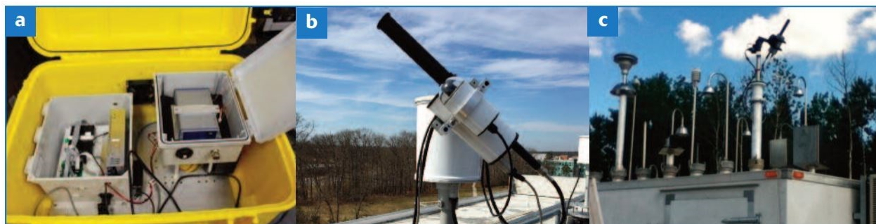
Figure 3.1: Pandora Ground-Based Spectrometer: (a) electronics box and the spectrometer; (b) 2-axis positioner with the telescope assembly; (c) deployment example on top of an EPA trailer [10].
