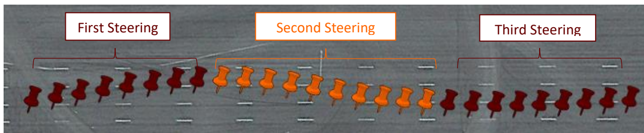
Figure 5-29. GPS results for a double lane change test via Google Earth. There are three steering actions in a DLC.
