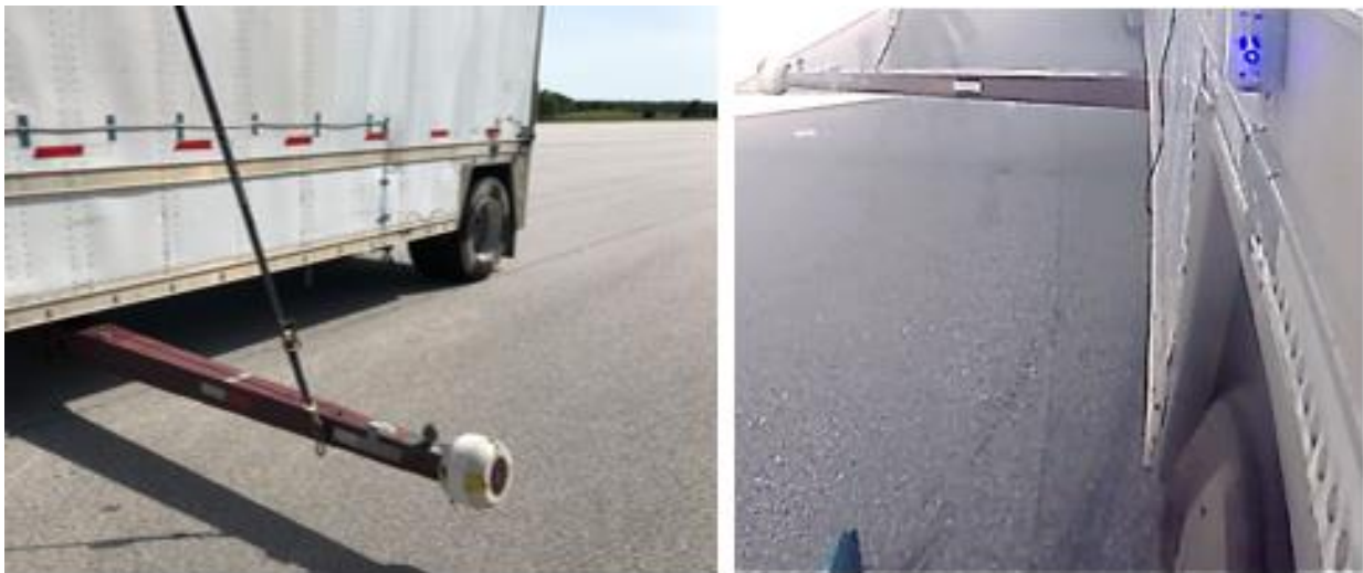
Figure 4-16. Outrigger wheel and vehicle wheel preparation.
