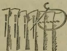
Fig. 5. Stitch on top side of wire.
