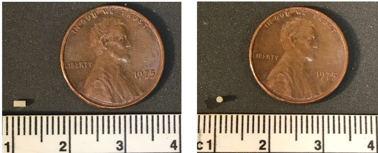
Figure 18: Final 2 mm height (left), 1 mm diameter (right) sample with a U.S. penny for size reference.
