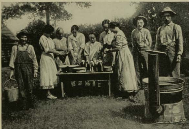
FIG. 55.—Canner made of tubs for outdoor use.
