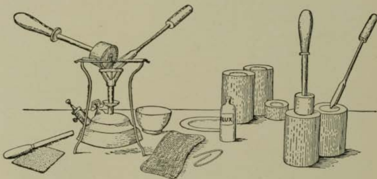
FIG. 45.—Heating tools, capping, and tipping.
