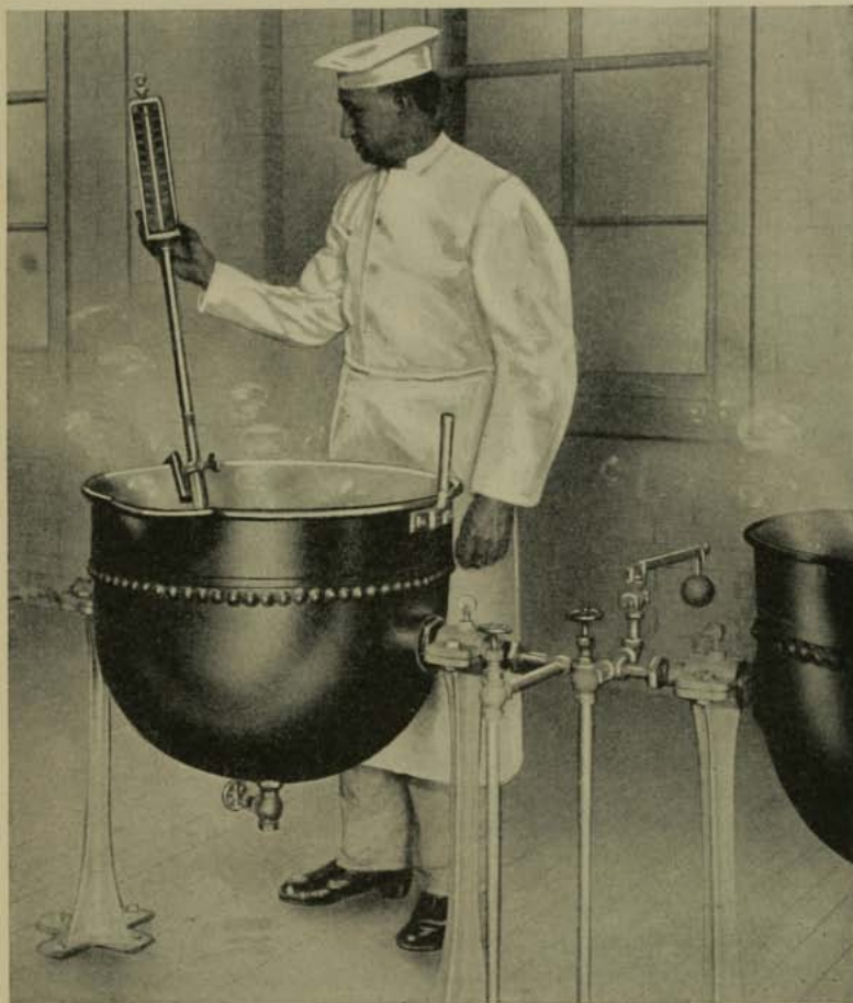
FIG. 95.—A steam-jacketed preserving kettle. (Heinz Company.)
