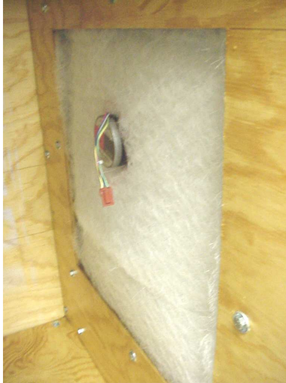
Figure 2.15: Filter material added to swirler inlet
