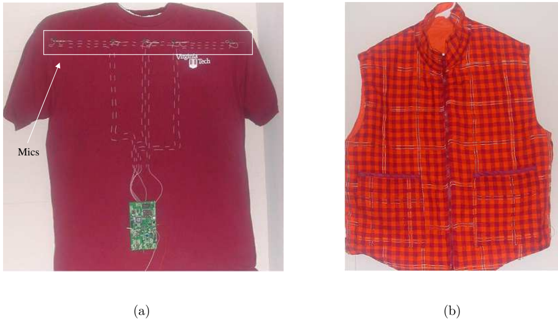
Figure 3.2: The Vest Beamformer is able to locate and distinguish between different audio sources.
