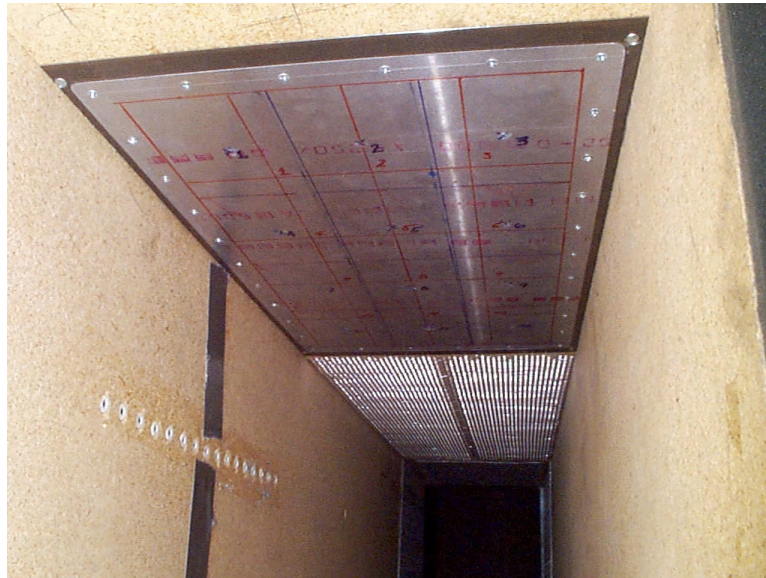
Figure 2.17: Sixteen microphones were mounted along the centerline of the tunnel side wall to determine the correlation of the turbulent flow.
