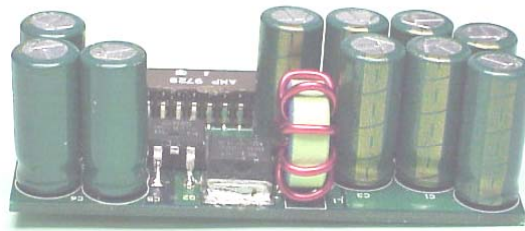
Fig. 1.8. 5V-input single-phase buck VR: (a) The schematic, and (b) a product photograph.
