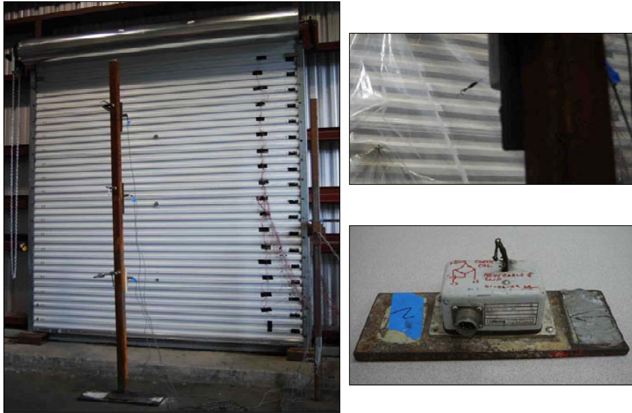
Figure 13. Wire pots were measure out-of-plane displacement
