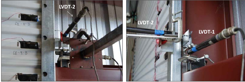
Figure 15. LVDT-1 and LVDT-2 measure jamb displacements
