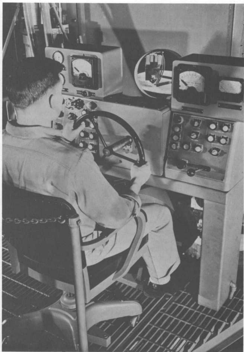
The operator views the cutting action through an arrangement of mirrors and steers the work to the saw. The simple wheel control coordinates the movement of the three power-driven tables. (Courtesy, The DoAll Company)
