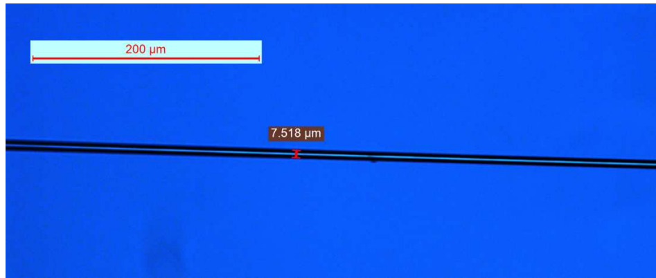
Fig. (6.5): (a) SHS measured for 10PAH/PB with phase-mismatching (blue line) and with QPM (red line), and (b) measured fiber taper diameter using optical microscope.
