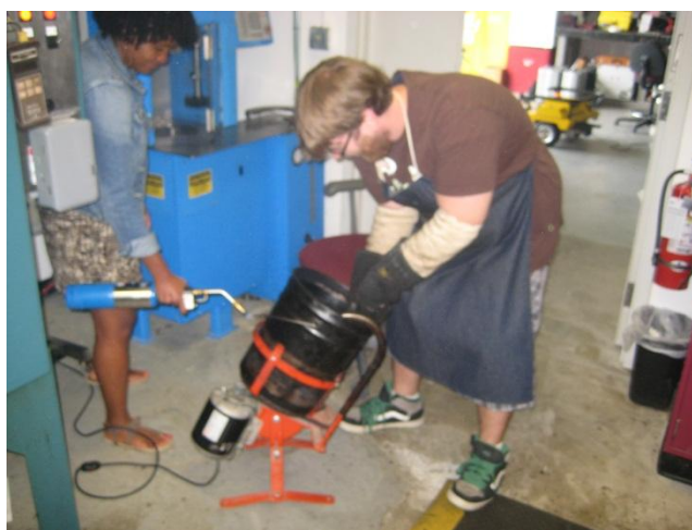
Figure 9. Using Propane Torch to Maintain Temperature
