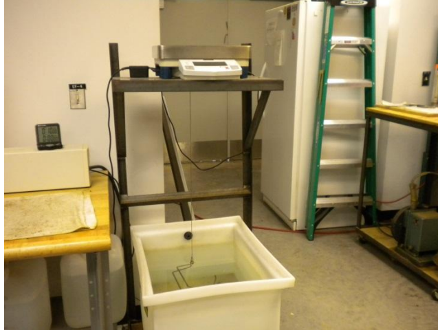
Figure 13. Gmb Equipment at VTTI
