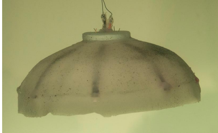
Figure 7-6. Artificial A.aurita with uniform bell and flap, in the relaxed configuration
