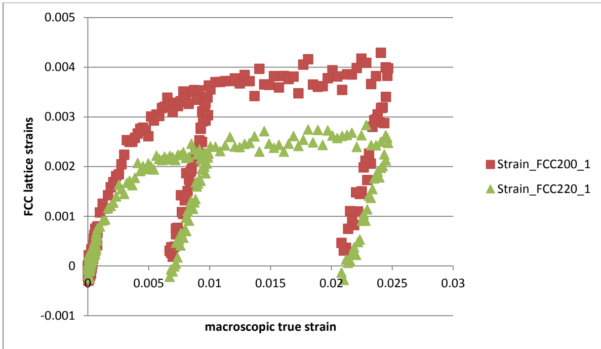
Figure F-17: True strain vs. longitudinal lattice strains for FCC planes in high Mn alloy (sample 3)
