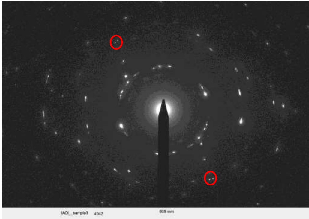
Figure 4-54: Evidence of twins in Diffraction Pattern (magnified)
