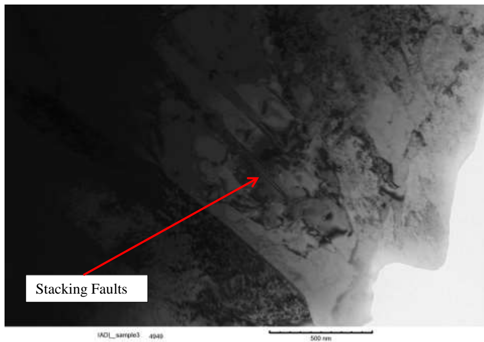
Figure 4-51: Stacking Faults in Austenite
