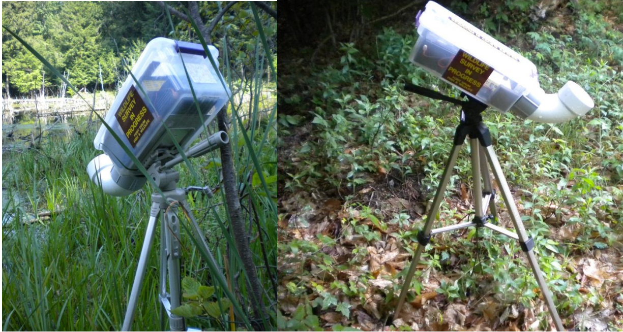
Figure 2.5 Passive acoustic sampling setup using Anabat detectors encased in weatherproof boxes mounted on 1.5 meter tripods at a 45° angle with polyvinyl chloride (PVC) tubes attached that contain a small hole in the bottom for water drainage, Fort Drum Military Installation, New York, summers 2011 and 2012.
