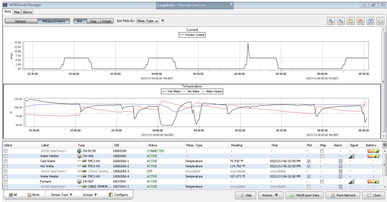
Fig. 32 Screenshot of HOBOnode Manager Used to Manage The Gas Water Heater Tank Data
