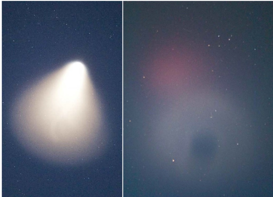
Figure 2.7: (left) Dust and neutral exhaust release and (right) dust ring and red lines emission. Figure reproduced from Bernhardt et al., 2011. Used under fair use, 2013.
