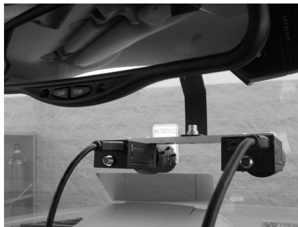
Figure 8. Luminance and color cameras.
