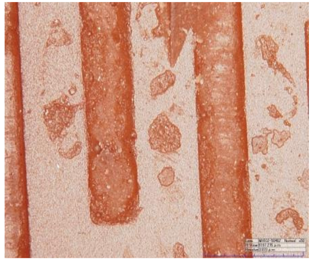
Figure 5.1: Chocolates examined under 50X magnification using a digital optical microscope. A & B unbloomed chocolates (top), C & D bloomed chocolates (bottom).
