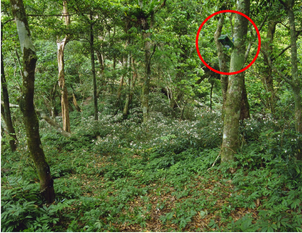
Figure 1.4. Camera set up for camera trapping in Tawu Nature Reserve and Twin Ghost Lake Important Wildlife Area, Taiwan, 2001-2004. Cameras (circled in red) were attached to a tree trunk facing downward to the trail or the intersection of trails at around 40-60 degree.
