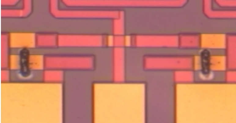
Figure 5.7: Laser trimmed traces to remove C_{r,add} .
