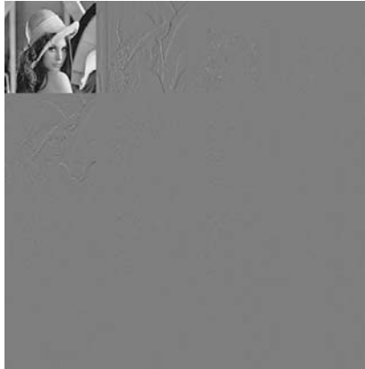
Figure 5.3: Transform coefficients of Lena image after one level of decomposition with the SA4 multifilter. Values near zero are shown in gray, with positive values increasing toward white and negative values decreasing toward black.
