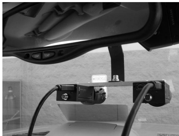
Figure 10: Luminance and Color Cameras
