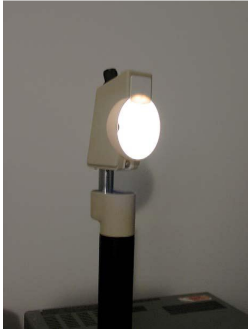
Figure 12: Brightness Acuity Tester (BAT)
