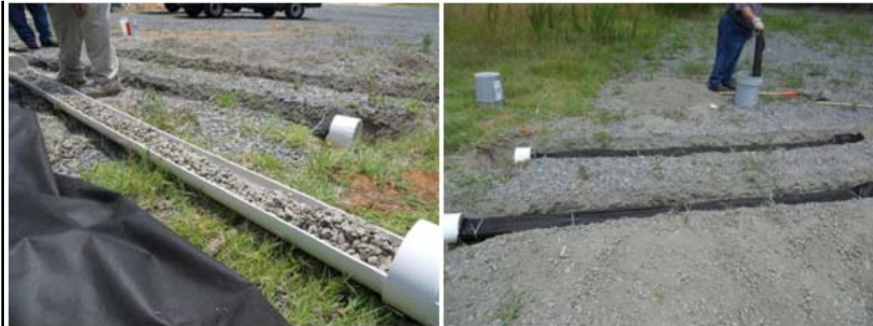
Figure 2. Plot 1: Lysimeters filled with aggregate ( left ), covered with landscaping cloth, and positioned 10 in beneath the soil surface ( right ).
