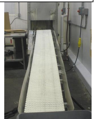
9. Steam tunnel: shrinks bags around prosciutto
