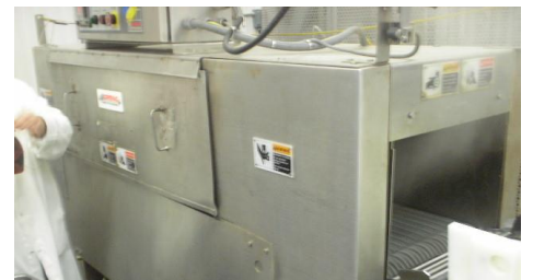
9. Steam tunnel: the bag shrinks around the product.
