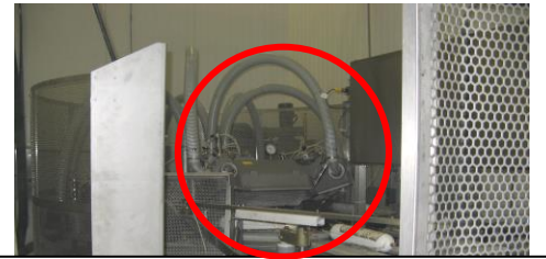
6. From the conveyor the product goes into the Cryovac machine in order to be sealed and the ink jet prints the date and lot # on product.
