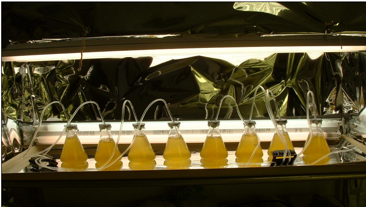
Figure 2: Reflective Mylar is used in enclosed growth chamber with optimal light and temperature control
