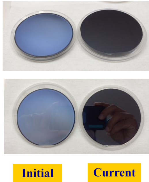
Fig. 13 Optical image showing epitaxial quality of GaAs grown directly on Si substrate by MBE. Left - initial direct GaAs-on-Si runs prior optimization, Right – surface quality of current optimized process-of-record (right) utilizing a sequence of LT/HT growth.
