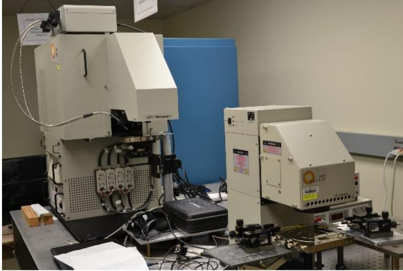
Fig. 4 Quantum efficiency and light/dark I-V measurement facility with the ADSEL group.
