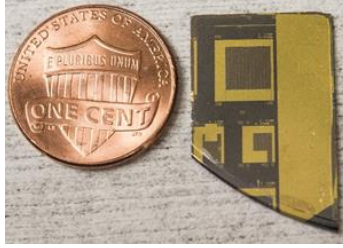
Fig. 3 Optical image of 0.5 cm 2 1J GaAs solar cell grown on Si substrate with both front-side metal contacts.
