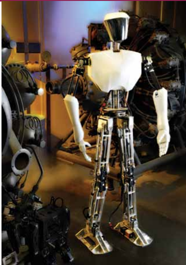
CHARLI (Cognitive Humanoid Autonomous Robot with Learning Intelligence) is the first untethered, autonomous, full-sized, walking, humanoid robot with four moving limbs and a head built in the United States. Built by undergraduate engineering students, CHARLI also can talk.
