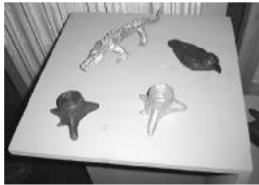
Finished castings in aluminum and brass
