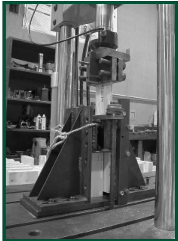
Test setup for analyzing the durability of wood-based composites sheathing connections following exposure to moisture content changes.
