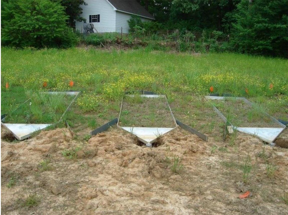
Figure 2: Close up photograph of one of the poultry litter plots showing the runoff collection apparatus.
