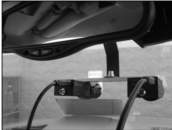
Figure 9. Photo. Luminance cameras mounted.
