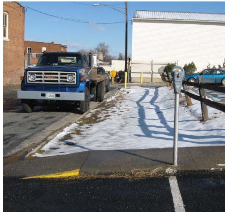
View down Goodwin street servicing Hill Hardware. Used for large truck parking and unloading. Grassy area serves as an infiltration trench and is accidentally parked on.
