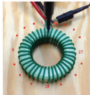
(a) Five turns model (b) Equivalent model with stray cap (a) Measurement setup Fig. 1 High frequency near-field stray flux explanation
