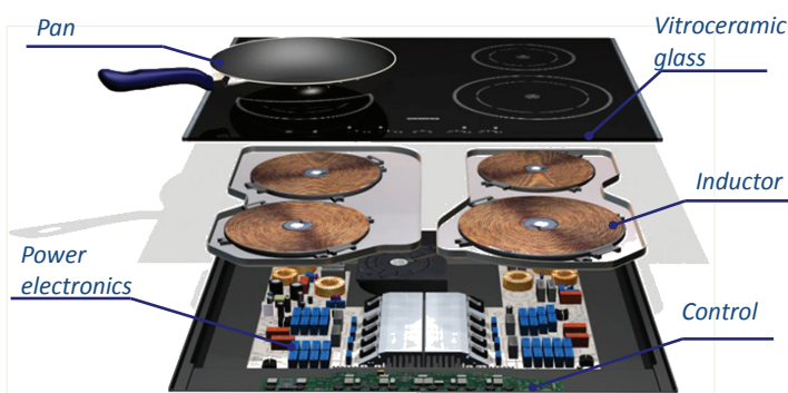
Fig. 1. Induction heating appliances: main parts of an induction heating cooktop.
