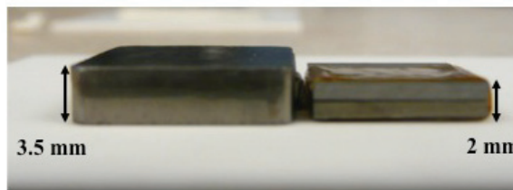
Figure 3. Dimension comparison between constant-flux inductor and a commercial inductor from Maglayers MMD-12CE-1R5M-V1.
