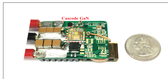
Fig. 2. Prototype of 5 MHz converter with cascode GaN switch.
